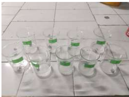
Fig. 2. Representative Images of Composite Samples Before Immersion in 3.5% NaCl Solution.
