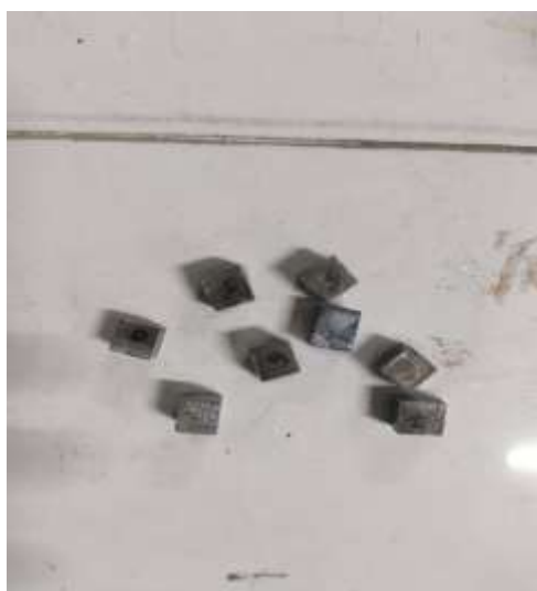
Fig. 2. Representative Images of Composite Samples Before Immersion in 3.5% NaCl Solution.
